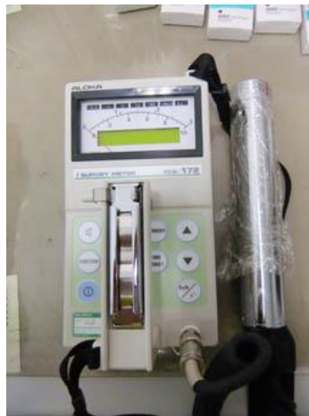
Fig. NaI(Tl) scintillation detector (with an energy-compensated Geiger–Müller tube)
