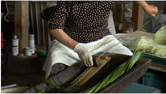
Fig. 1 Ohiki (fiber extracting) process in Showamura, Fukushima prefecture (photo by Tokyo National Research Institute for Cultural Properties)
