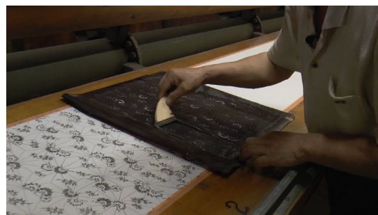
Fig. 5 Printing using a stencil (photo by Tokyo National Research Institute for Cultural Properties)
