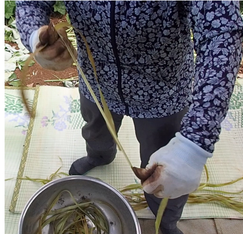
Fig. 3 Ohiki (fiber extracting) process using a mimigai ( Haliotis asinine ) (photo by Tokyo National Research Institute for Cultural Properties)
