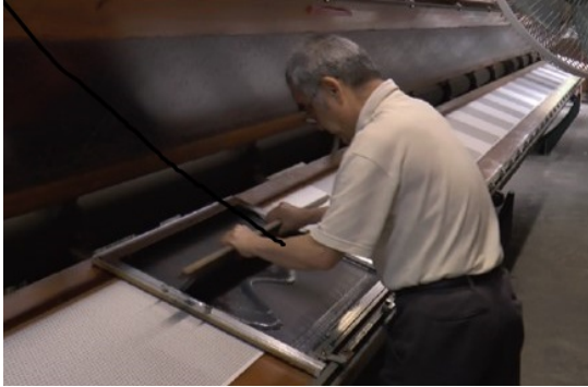
Fig. 6 Printing using a screen (photo by Tokyo National Research Institute for Cultural Properties)
