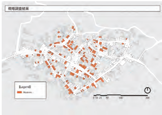
Fig.6-8 Location of the traditional buildings that have suffered moderate level damage in the south area
