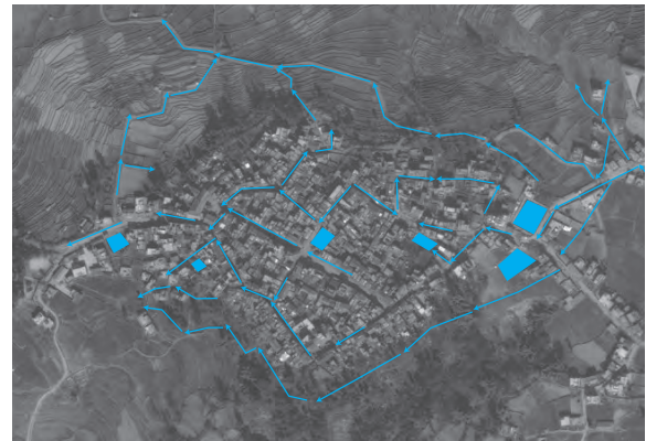
Fig.6-19 Traditional drainage system inside and periphery of Khokana
