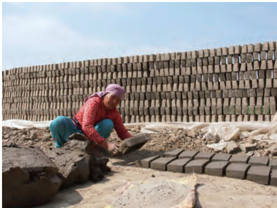
Fig.3-8 Female worker manufacturing dātiapā bricks
