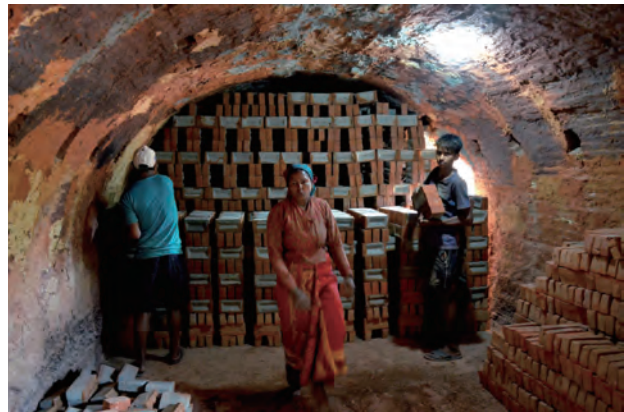
Fig.3-9 Taking out dātiapā bricks from the brick kiln
