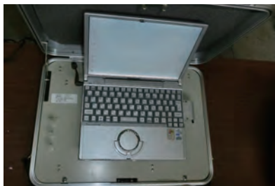
Portable vibration monitoring system (SPC-51)
