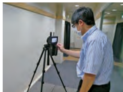
国宝高松塚古墳壁画仮設修理施設の見学通路における微粒子測定 Measuring fine particles in the visitors' corridor of the Takamatsuzuka Tumulus
