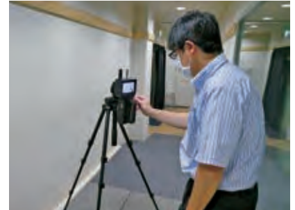
国宝高松塚古墳壁画仮設修理施設の見学通路における微粒子測定 Measuring fine particles in the visitors' corridor of the Takamatsuzuka Tumulus
