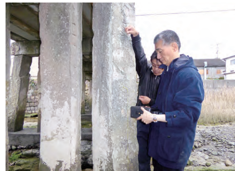
重要文化財・祇園橋における石材の水分量調査 Investigation of the moisture content of stones constituting the Gionbashi Bridge, a nationally designated important cultural property
