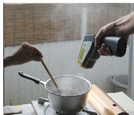
漆を加熱して硬化させる堆錦技法の非接触温度測定調査 Measurement of urushi temperature by infrared radiometer in tsuikin technique, a kind of thermal polymerization of urushi
