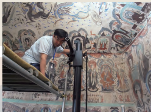
ハンドヘルド蛍光X線分析装置を用いた敦煌壁画の分析調査(中国) On-site analysis of the painting materials of mural paintings at Mogao Grottoes, Dunhuang, China, using a handheld X-ray fluorescence spectrometer
