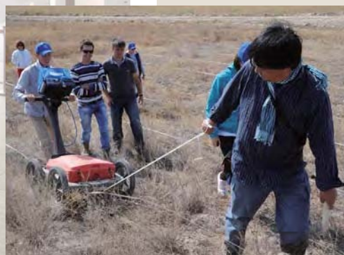
地下探査実習(カザフスタン) On-site training using ground-penetrating radar (Kazakhstan)
