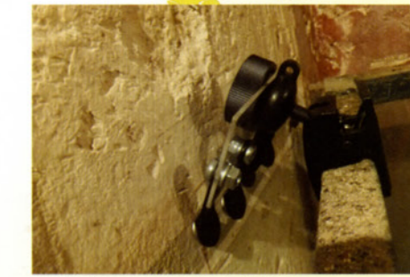
中国陝西省の古墳における壁画含水量の測定 Measurement of water content on the mural paintings of a tumulus in Shaanxi province, China
