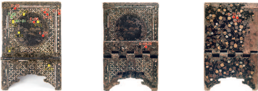
Fig. 4 Sampling and measurement location on Lectern (1) ▲ (triangle, T) denotes the digital microscope observation points; ● (circle, C) represents the XRF measurement points; and ■ (square, S) indicates the sampling locations utilized for digital microscopy, SEM observation, cross-sectional observation, SEM-EDS, and THM-GC/MS analysis.
