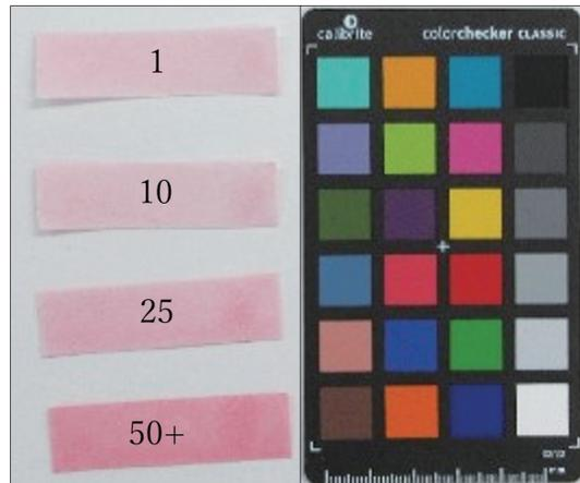
**Figure 4** Iron(II) ion presence reference strips made in accordance with CCI's Iron(II) ion test strip colour chart<sup>20</sup>
