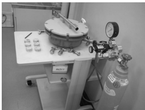
Fig.3 Pressure plate experiment set for tuff breccia
