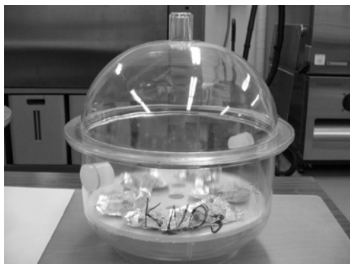
Fig.4 Saturated salt solutions experiment set for tuff breccia
