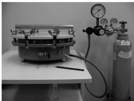
Fig. 5 Plate pressure experiment set up
