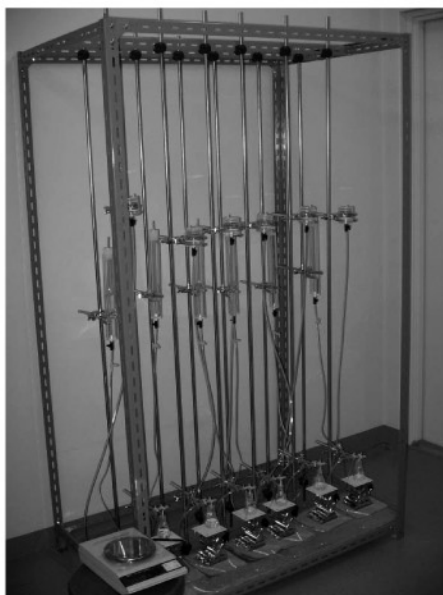
Fig. 4 The water hanging columns experiment set up
