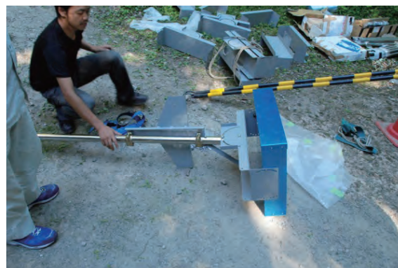
Fig.16 UV-C irradiating system for Kumano Stone Buddha
