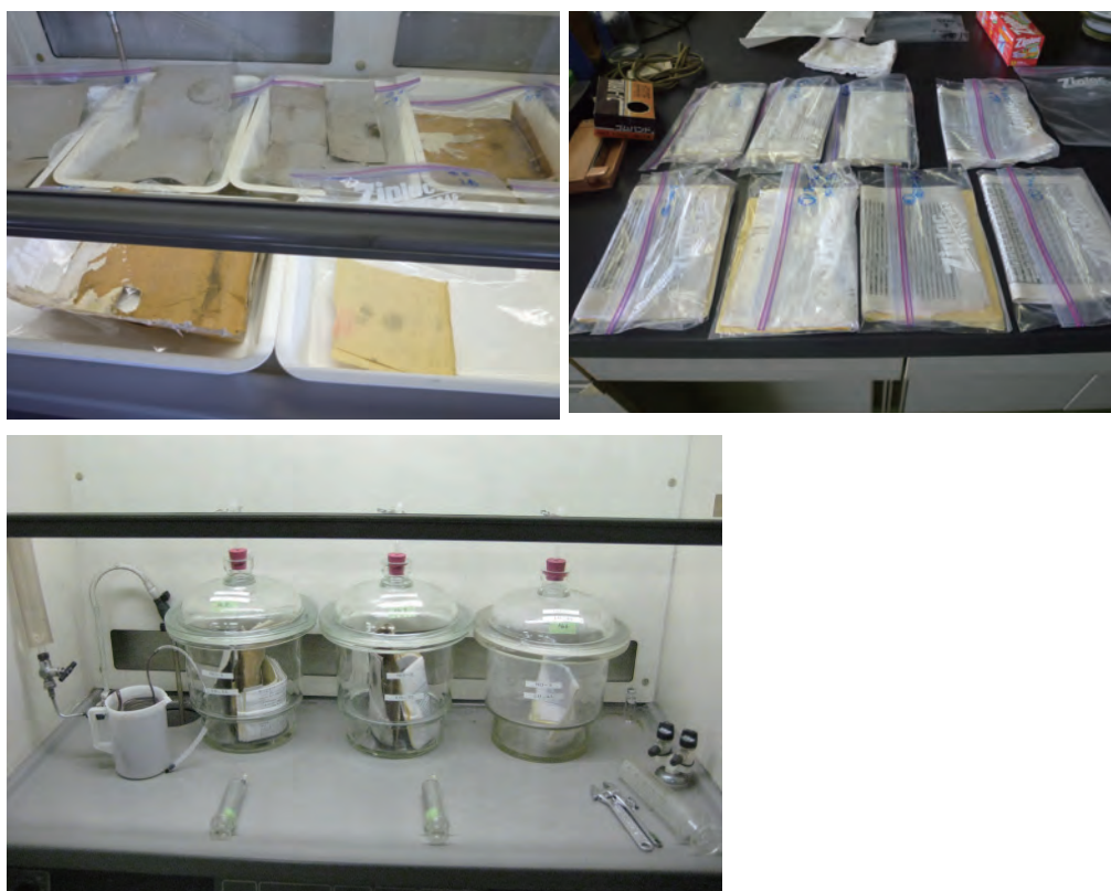
Fig.19 Experiments of fungicidal fumigation of seawater-soaked, wet or dried paper or documents.
