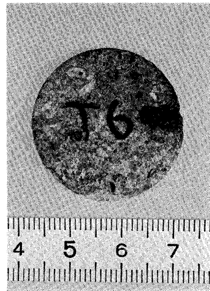
図-5 凝灰岩試料（シリコン樹脂処置） Fig. 5 Sample (Tuff-treated by silane)
