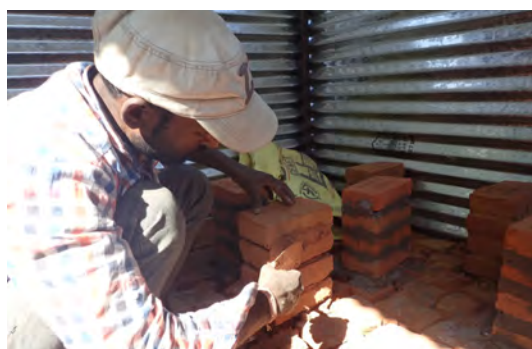
Fig.2-3-1 Making specimens for structural material testing
