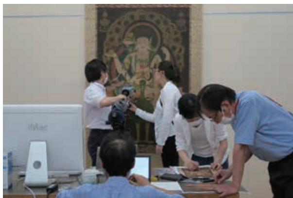
国宝孔雀明王像の蛍光X線分析の様子(東京国立博物館) Analysis of the Painting of Kujaku-myō-ō by X-ray fluorescence spectrometry (Tokyo National Museum)
