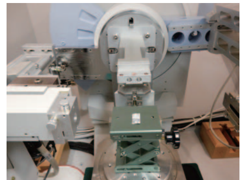
金属試験片のX線回折分析 X-ray diffraction analysis of a metal test piece
