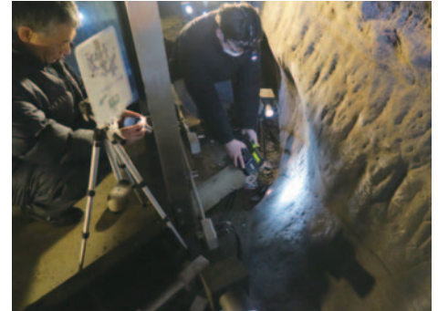
国指定史跡・フゴッペ洞窟の壁画面での岩体水分量計測 Measurement of the water content of the petroglyph of Fugoppe Cave, a national historic site
